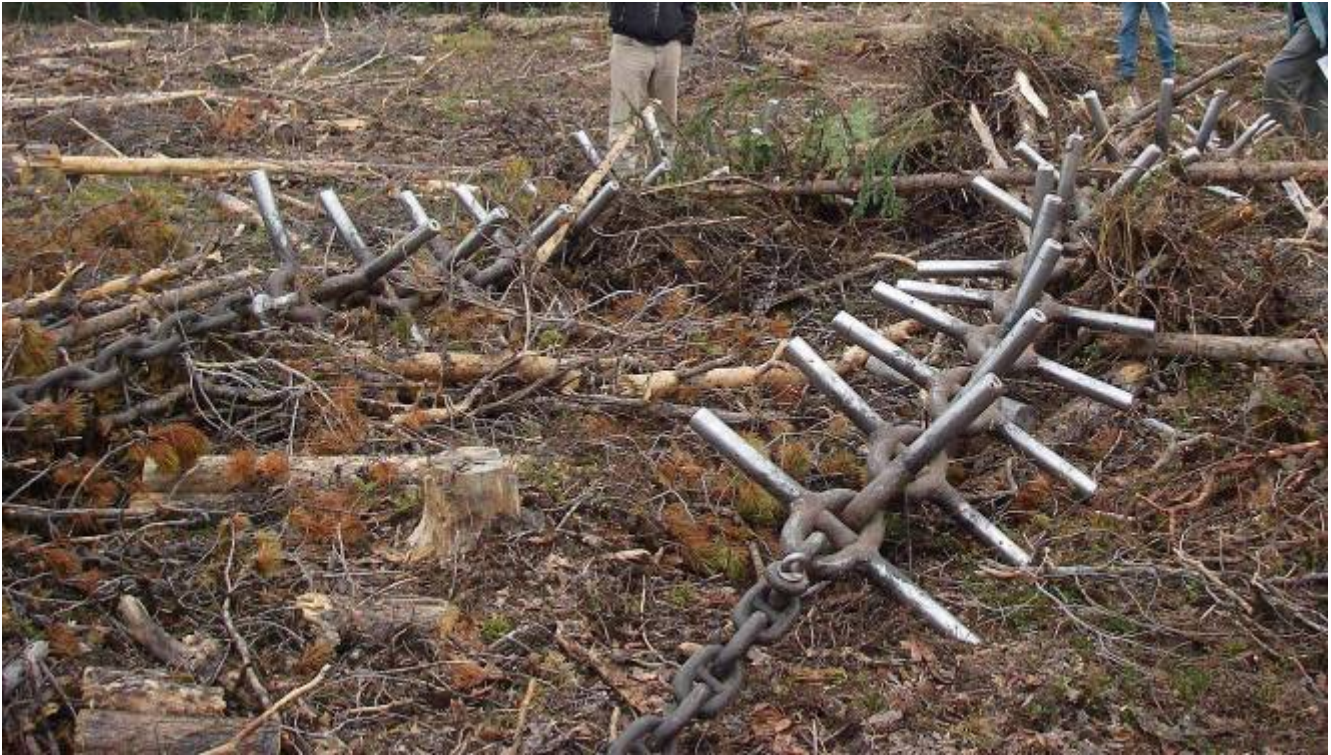
Figure 2: Drags used for drag scarification to promote natural regeneration.
