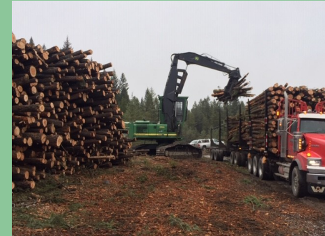
An example of a high level of utilization where logs that are small diameter and short in length are hauled. The above truck was loaded with several hundred logs.
