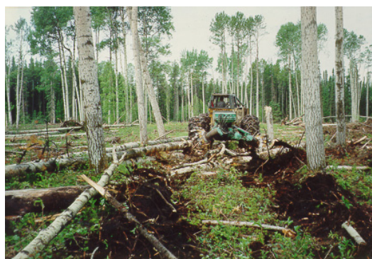
Disc trencher scarifying cutunit to prepare planting spots.
